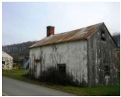
Fig. 1. This 200 year old log cabin is similar to the kind of small log house that Gucker would have built. The exterior of even this small house was weather boarded with vertical boards. Photo by M. Falconer 2010.
