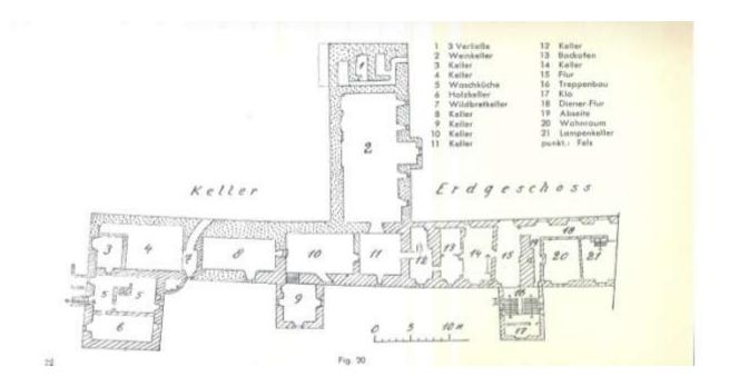
Fig. 2. Castle Wittgenstein, cellar level, showing part of today's structure. (Note that the orientation here is different from that of Fig. 1, which has North at the top. Here North is to the right.) The thicker, dotted cellar walls are of earlier date than those with hatching.
